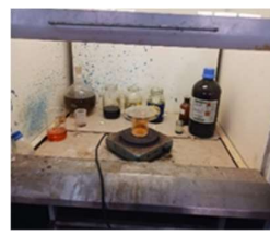
Plate 4. Fume chamber for digestion of honey sample using aqua regia before mineral analysis.
