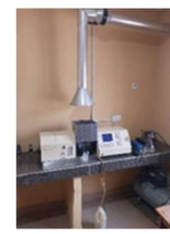
Plate 5. Shows Atomic Absorption Spectrometry (AAS) used for mineral and heavy metal analysis.
